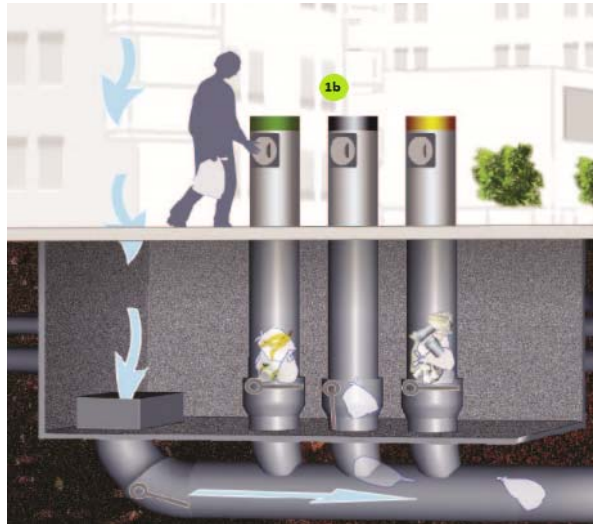
Figure 5 – Outdoor waste inlet at ground level
